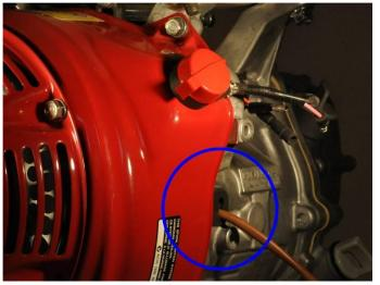
After mounting the coil the red hood can be put back
