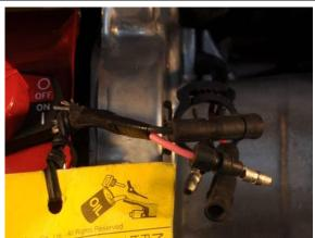
Disconnect the wires of the power switch.
