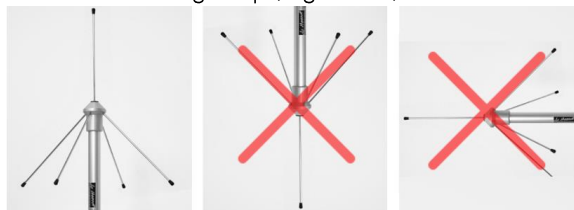
Figure 14: good/bad example: direction of the antenna
