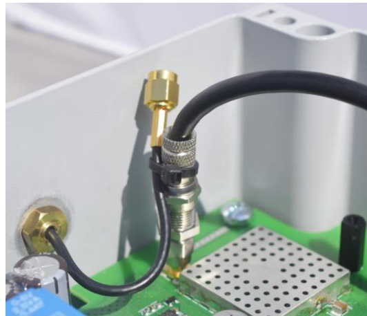
Figure 10: inside view, former antenna cable secured
