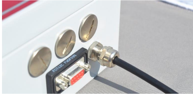
Figure 5: bottom view, cable gland with fed antenna cable
