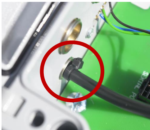
Figure 11: inside view, a tie wrap is attached to the antenna cable as a cable strain relief
