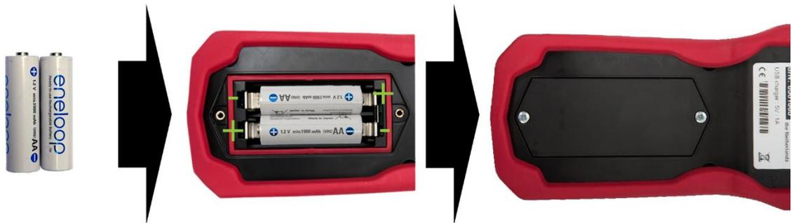
Figure 10 Battery insertion
