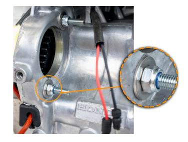
Pull the **brown** cable of the Xtra.Universal Power Coil through the cable guide of the engine. Leave as little cable in the flywheel housing as possible.
