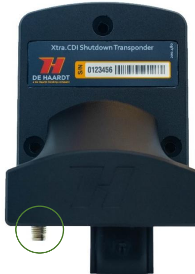
Figure 6: Xtra.CDI Shutdown Transponder network port
