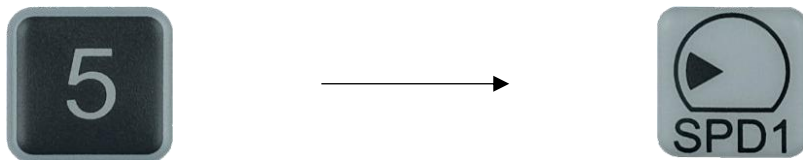
Figure 25 - Go-kart number adjust speed sequence to set go-kart number 5 to SPD1 .
