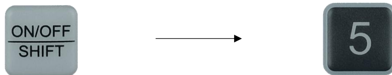
Figure 26 - Extra speed sequence, sets SPD5 . (Electro 8 Speed only)
